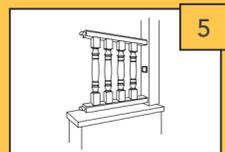
With the bottom bracket temporarily in place, offer and locate the front post to the spindle and rail unit (Fig 6a). Mark the position of the Porch Canopy to the top of the front post (Fig 6b) allowing for either:
